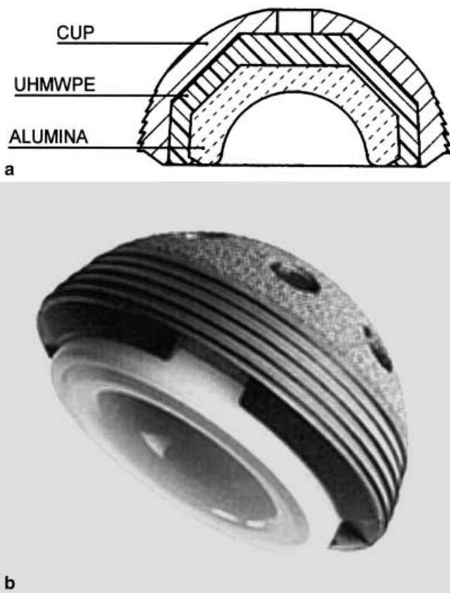
**Fig.1** a Diagram of the Contact acetabular component section showing the three different layers. b The socket as a whole
