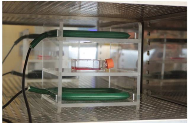
**Fig. 1** Pulsed electromagnetic field device used for all the experiments, placed in a 5 % CO<sub>2</sub> and 37 °C incubator. TCs seeded in T25 culture flasks (like in the picture) or in 24-well plates were placed between the pair of coils so that the plane of the coils was parallel to the culture layer. The peak values measured between the two coils in air had a maximum variation of 1 % in the whole area in which the culture flasks were placed. Cells were exposed to PEMF for 4, 8 or 12 h
